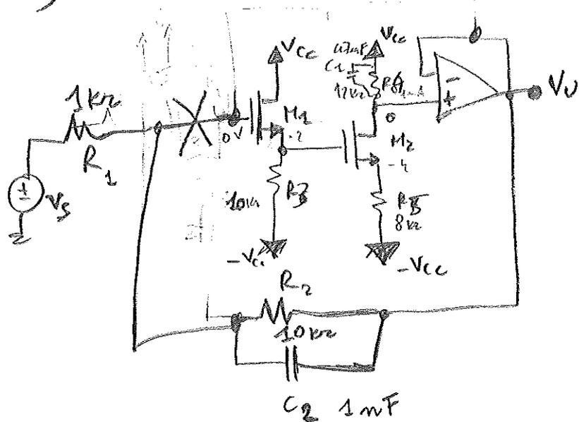
Se  $V_U = 0 \Rightarrow$  Per il CCV  $V_{op}^+ = V_{op}^- = V_U = 0 = V_{D2} = 0V$
