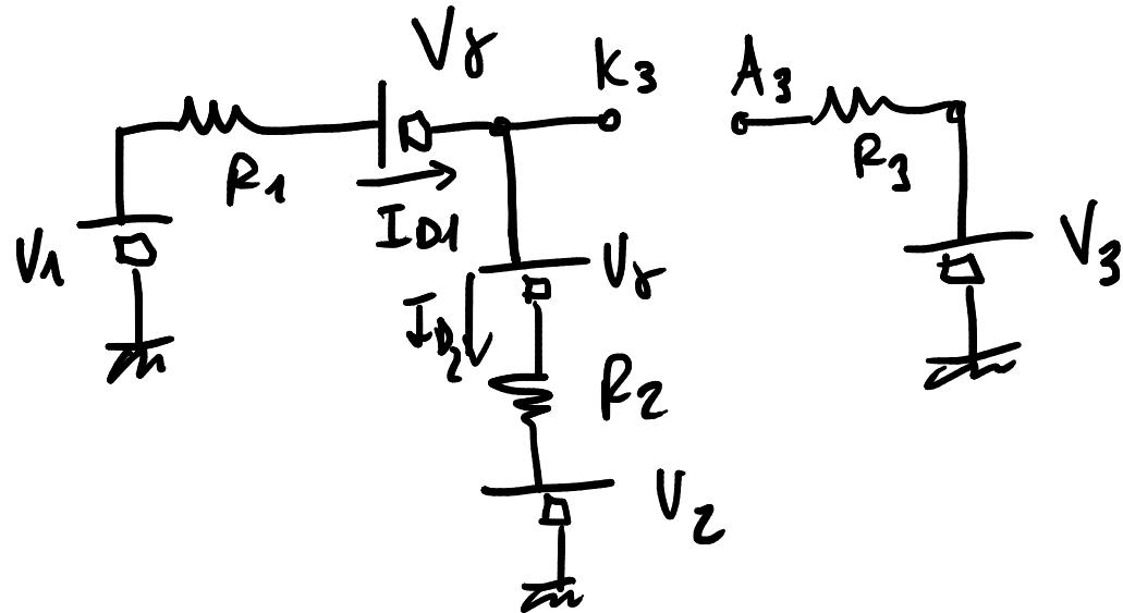
$$I_{D1} = I_{D2} = \frac{V_1 - V_2 - 2V_F}{R_1 + R_2} = 3,3 \text{ mA} > 0$$
