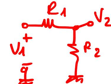
$$V_2 = \frac{R_2 V_1}{R_1 + R_2}$$
