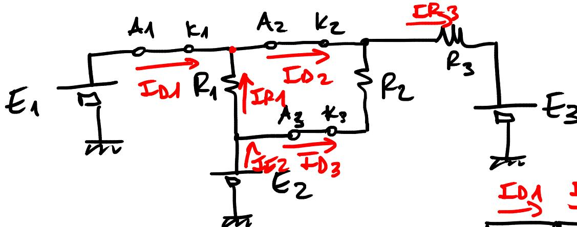
$$I_{E2} = \frac{E_2 - E_1}{R_1 || R_2} \approx 5,5 \text{ mA}$$
