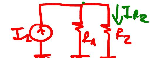
$$IR_2 = \frac{R_1 I_1}{R_1 + R_2}$$
