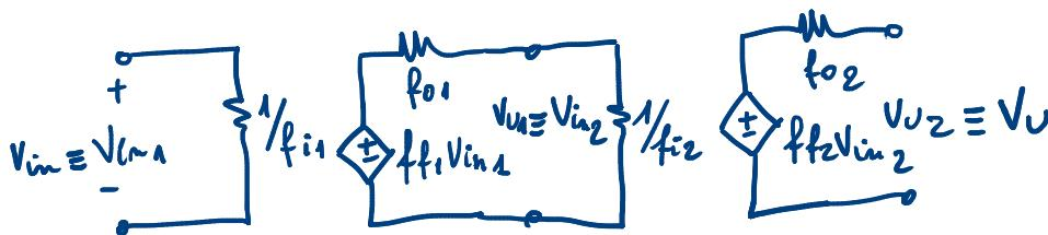
$$V_U = f_{f2} V_{in2} ; V_{in2} = \frac{1/f_{f2}}{f_{f1} + 1/f_{f2}} f_{f1} V_{in1}$$
