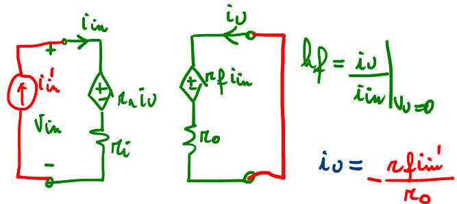
$$r_f i_m + r_o i_o = 0 \quad i_o = -\frac{r_f}{r_o} i_m$$
