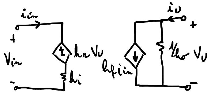
$$\left\{ \begin{array}{l} i_v = h_f i_{in} + h_o V_u \\ V_{in} = h_r V_u + h_i i_{in} \end{array} \right.$$
