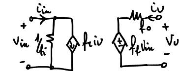
$$f_f = \frac{\bar{V}_o}{V_{in}} \Big|_{V_o=0}; \quad f_o = \frac{\bar{V}_o}{V_{in}} \Big|_{V_{in}=0}$$
