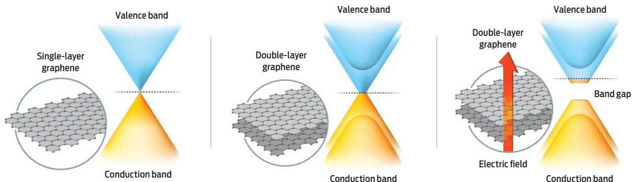
**BREAKING SYMMETRY:** The existence of an energy gap between the conduction and valence bands of a material is what makes it possible for it to act as a semiconductor. In both single-layer and double-layer graphene [left and middle], the valence and conduction
